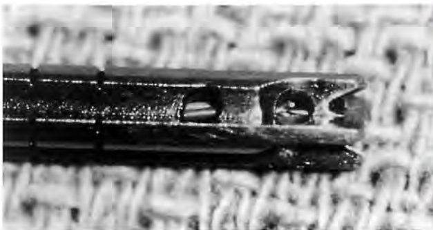
Figure 7. The exposed measuring portion of the thermocouple comes in contact with the bur tip.
